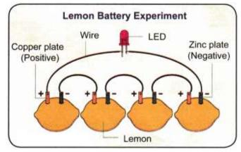
The first iron nail is to be connected to the negative terminal of the LED, and the last copper strip to the positive terminal of the LED. The LED will glow to show that the Voltaic cell is ready.
